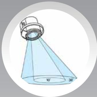
Interchangeable lamps can be switched from spot lighting to flood lighting.
